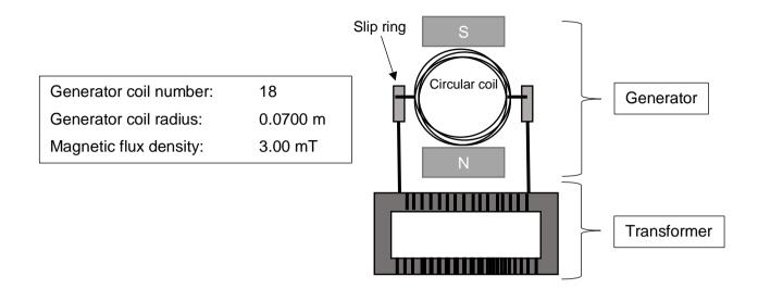
The demonstration generator is not capable of a high voltage output. To increase the output voltage, the demonstration generator was connected to a transformer. The primary to secondary windings ratio was 1:53, resulting in an rms output voltage of the transformer of 2.36 V.
